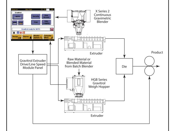
**Depicted above:** a complete Gravitrol system (featuring an EXB2 Operator Station, an HGB Series Weigh Hopper, an X Series 2 Continuous Gravimetric Blender and a multi-extruder drive/line speed module panel controlling a simple coextrusion application). Information is subject to change without notice. Use only certified drawings for construction purposes.
